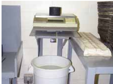
Weighing specimen to Determine G_{mb}
